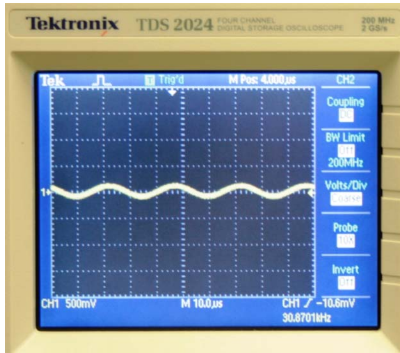
Fig.6-5: Received signal in air at a distance of 40cm.
